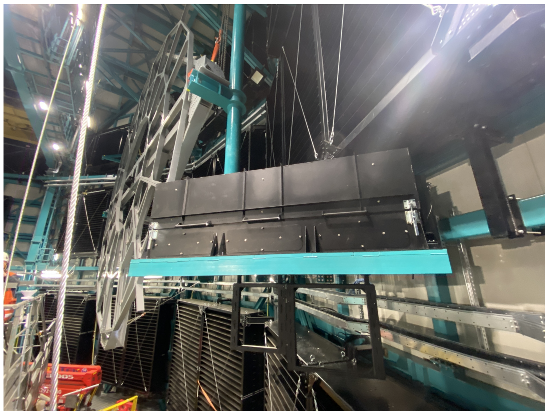
FIGURE 2: Image of the laser box, containing the Ekspla tunable laser, which was installed on the dome on November 21.
