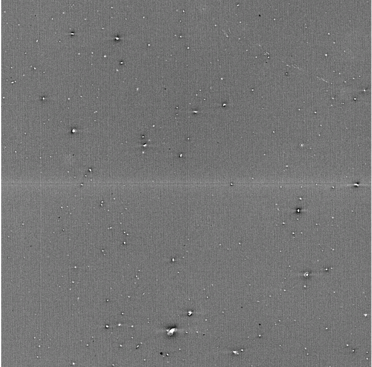
FIGURE 4: A view of detector R22_S10 in y-band, which has a large number of less significant vampire pixels.
