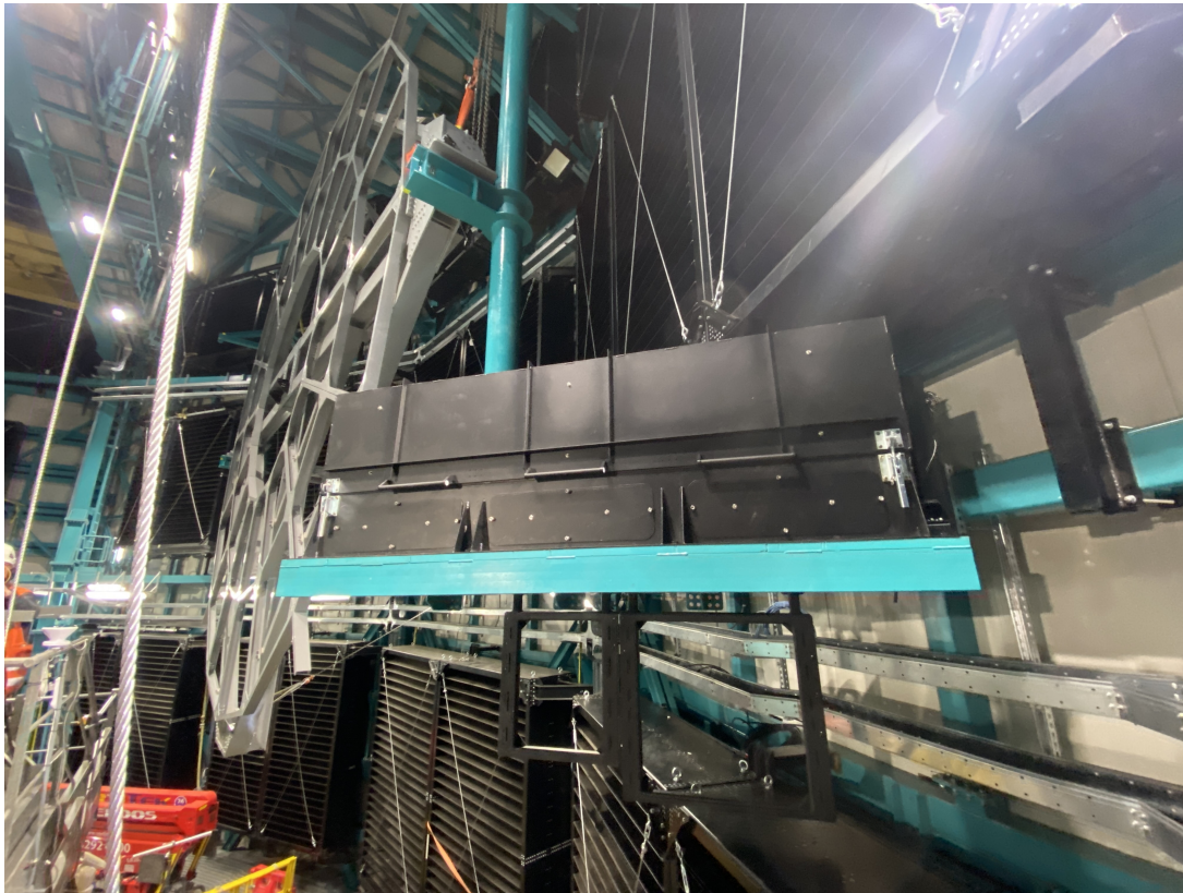
Figure 30: Image of the laser box, containing the Ekspla tunable laser, which was installed on the dome on November 21.
